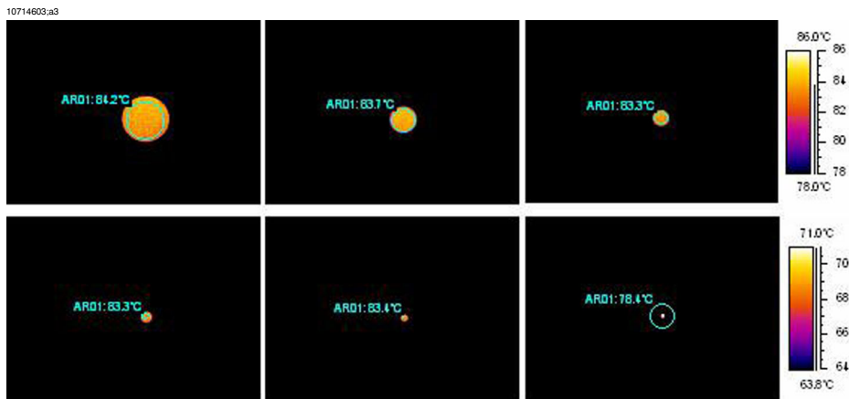
Figure 7.20 Temperature readings from a blackbody at +85°C (+185°F) at increasing distances (24° lens)
