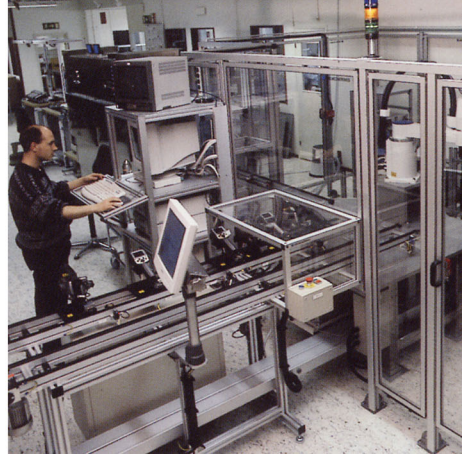
Figure 3.6 LEFT: Testing of IR cameras in the climatic chamber; RIGHT: Robot for camera testing and calibration
